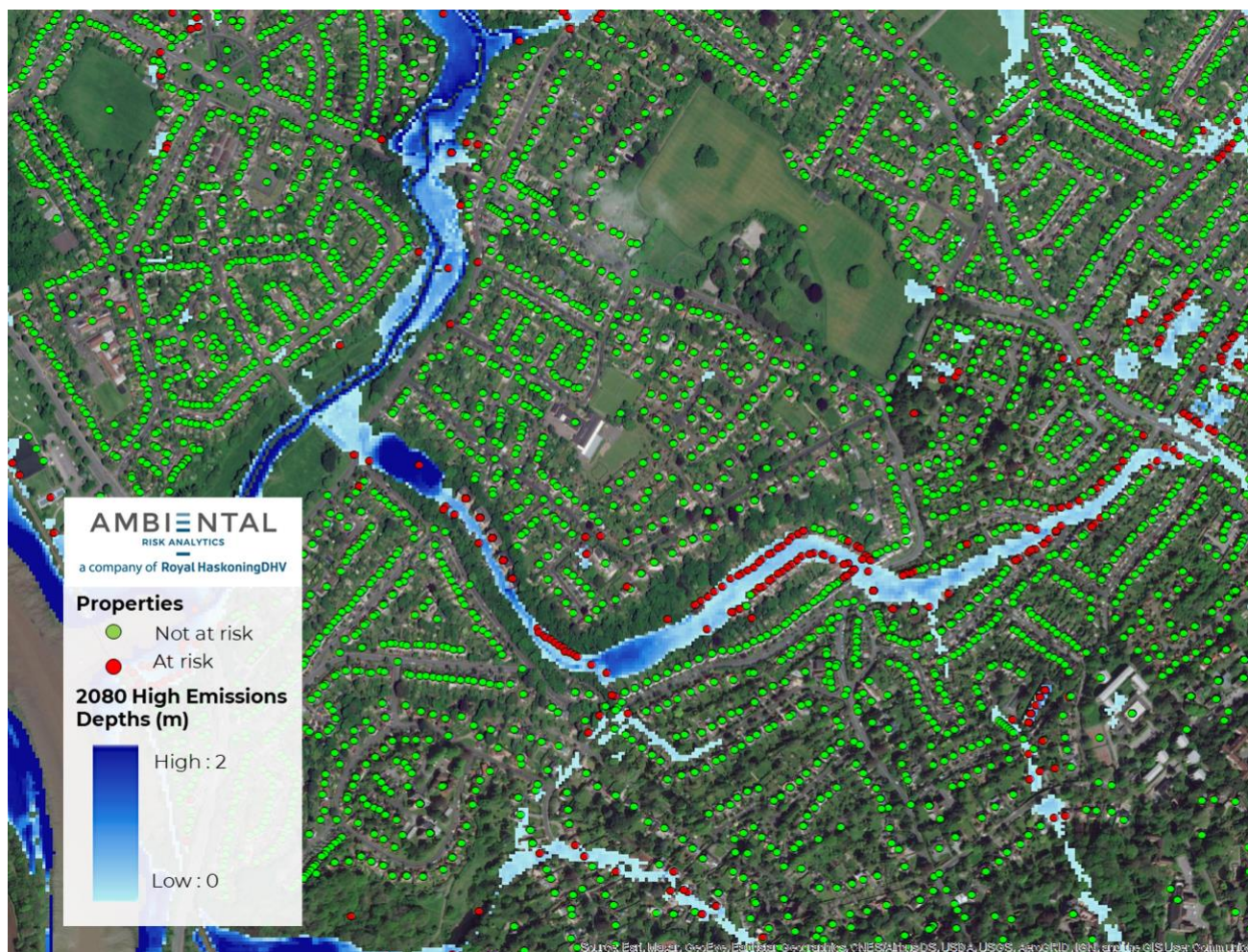
Figure 3. Extract of Ambiental's FloodFutures in Bristol showing pluvial flooding in the 2080s under the High Emissions scenarios
